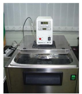
Picture on the left shows the Precision PID Temperature controller water bath for the Calibration Laboratory Standard.
